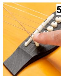
Push the pin into the bridge then pull the string taut locking it in place.
