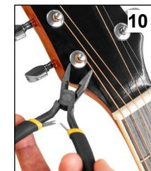
Carefully cut off any excess string using wire cutters or a special tool.
