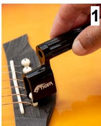
Pull straight upwards with a pin puller to remove the bridge pin.
