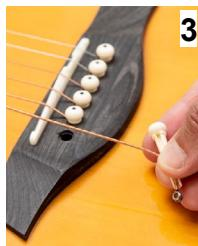
Position the string in the groove in the pin.
