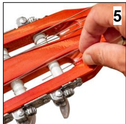
5 Pull the string through the hole in the tuning peg.
