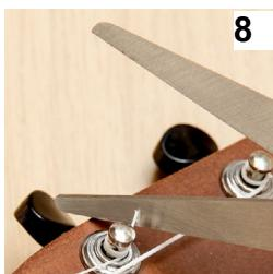
Pull the string through the hole in the tuning pin.
